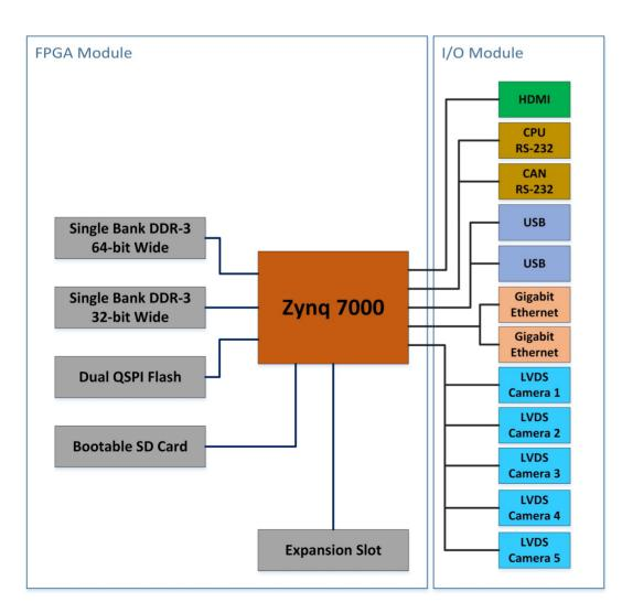
The functionality of the EM-ZynqBox will be extended by additional IP-Cores, e.g. for advanced Image Processing and rugged fanless variants.
