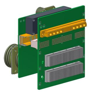
Internal I/O is routed from the backplane to the front panel connectors by means of a solid-state I/O transition module. This design philosophy, which was pioneered by Aitech, provides higher reliability and better signal integrity than harnessing, and is lower in cost. Designed with a built-in handle for convenient handling, the A191 is equipped with brackets and captive screws for convenient hard mounting.
