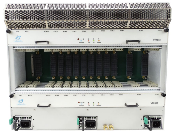
Figure 5: VTX661 Chassis Layout – Rear
