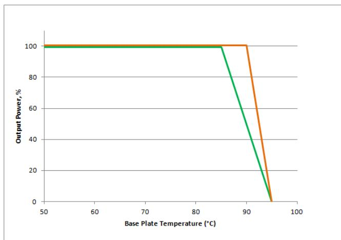
Thermal derating Output Power vs. temp at module cover.
